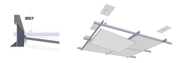
$\label{eq:Step2} Step\ 2$  Proceed with placing the remaining panels.
